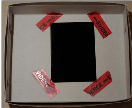
Figure 6. The mid-sized gel lifts may be secured inside 8.5” x 11” office paper or standard file folder cardboard boxes. Secure the corners of the gel lift to the bottom of the box using evidence tape.
