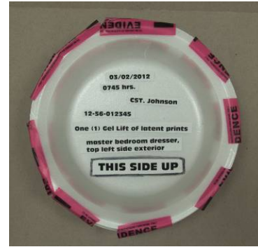
Figure 3. Secure the 'clam shell' using evidence tape and record the case information on the container.
